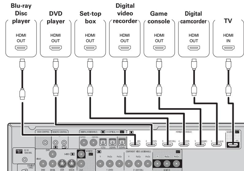
Connecting an HDMI-compatible device
