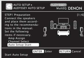
Here, we explain setup using the example of 5.1-channel speaker playback. For settings other than 5.1-channel surround, select "Amp Assign" and perform step 3 to 4 of "Set up speakers" (page 36). If unused channels are set with "Channel Select", measuring time can be shortened. For setting, perform steps 5 to 9 of "Set up speakers" (page 37).
