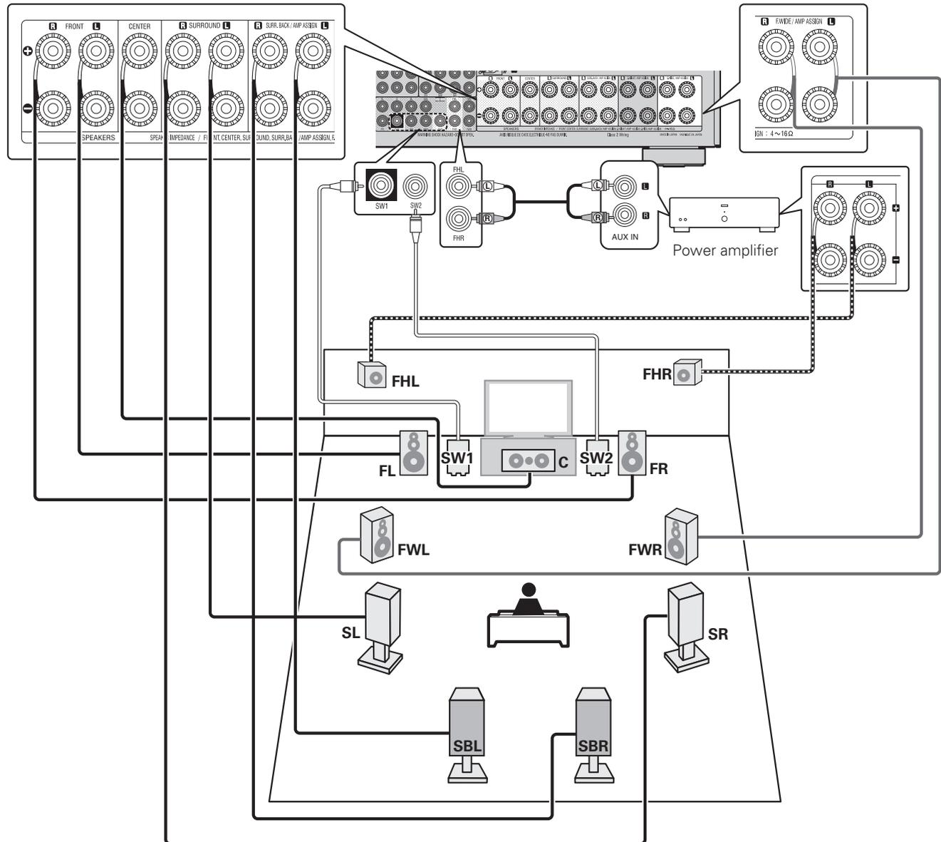
\* You can also change the PRE OUT connector for connecting the power amplifier to the Front channel using the "Amp Assign" – "Ext. Amp" settings (page 95). Change the setting in accordance with your preference.
