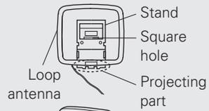
**2** Insert the projecting part into the square hole in the stand.
