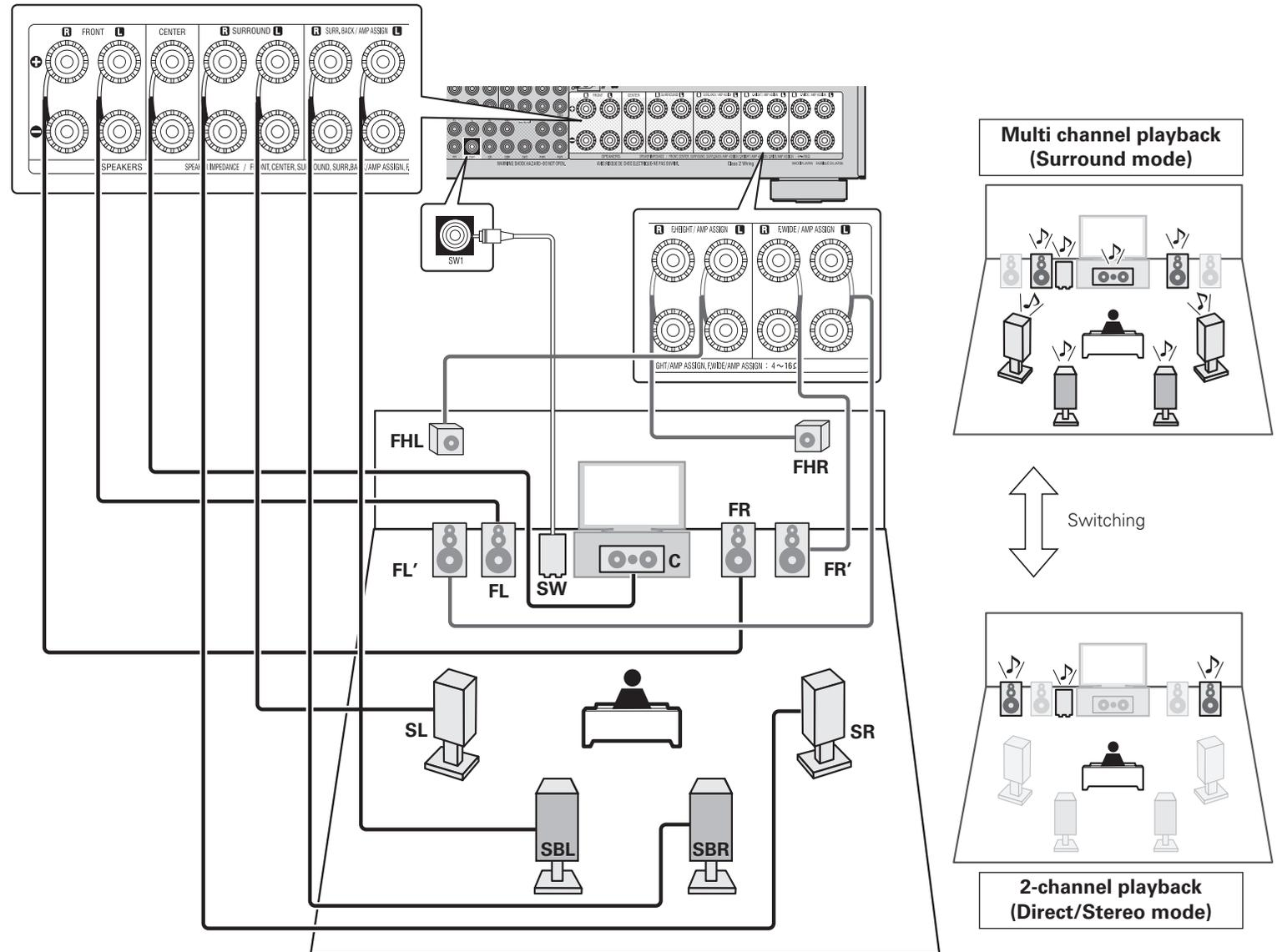
\* You can also change the 2-channel playback front speakers to SURR.BACK/AMP ASSIGN or F.HEIGHT/AMP ASSIGN speaker terminals using the "Amp Assign" and "Assign Sp." settings (page 95).
