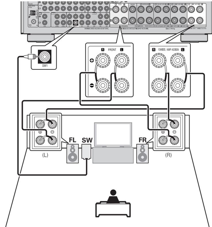
\* You can also connect the front speakers for bi-amp connection to SURR.BACK/AMP ASSIGN or F.HEIGHT/AMP ASSIGN speaker terminals using the "Amp Assign" – "Assign Sp." settings (page 95).
