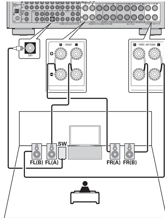
\* You can also connect the Front B speakers to SURR.BACK/AMP ASSIGN or F.HEIGHT/AMP ASSIGN speaker terminals using the “Amp Assign” and “Assign Sp.” settings (page 95).
