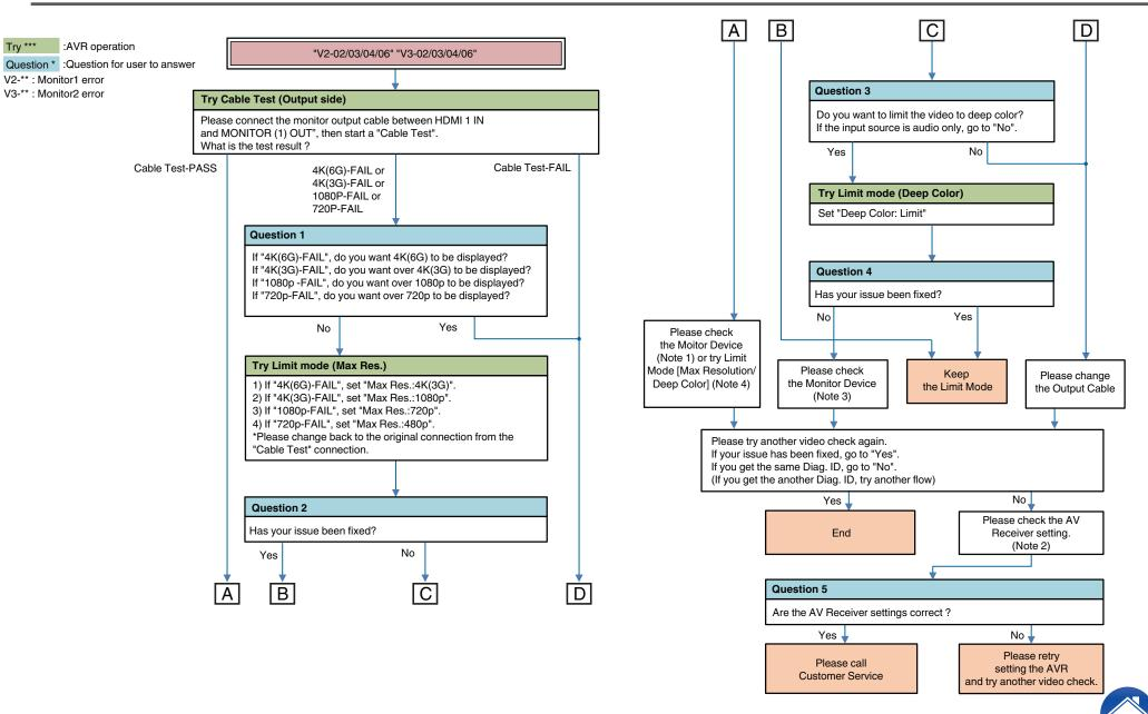
**Description "V\*-02"**: Miscommunication with Monitor at output terminal (4K60 output setting error).
