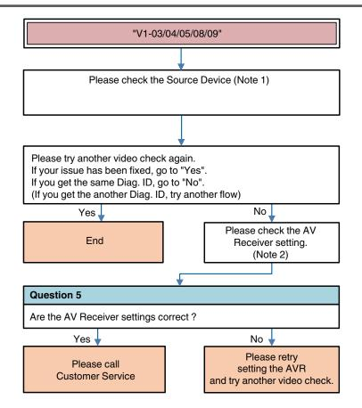
**Description "V1-03"**: Cannot detect the HDMI signal from the source device at the AVR input terminal (TMDS Rx PLL Lock, but SCDT(CKDT) OFF).
