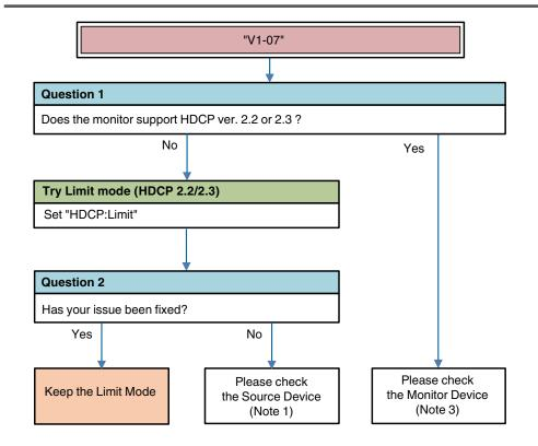
**Description** "V1-07": HDCP2.2 or 2.3/Stream ID Type mismatch (ie. Stream ID = 1, but Monitor's HDCP = V1.4).
