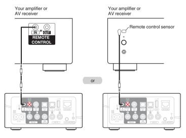
Connecting the IR control cable (IR Direct cable/IR Emitter cable) to the Trigger
