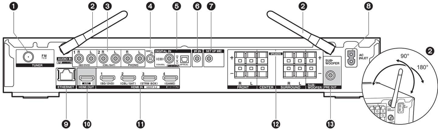
1. TUNER FM 75Ω jack: Connect the supplied antenna.
