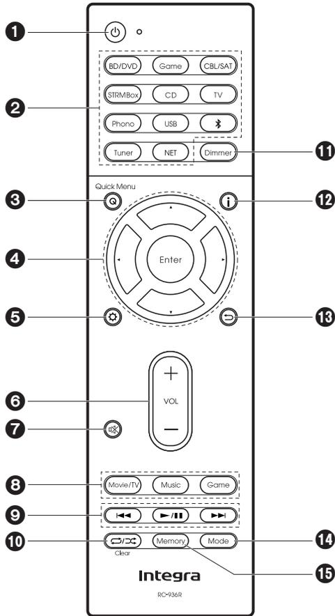
1. button: Turns the unit on or into standby mode.
