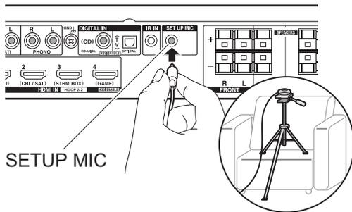
When putting the speaker setup microphone on a tripod, refer to the illustration when putting it in place.
