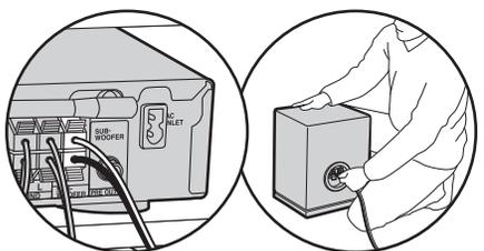
Make sure the exposed wires of the speakers do not stick out of the speaker terminals when connecting. If the exposed wires of the speakers touch the rear panel or the + and – wires touch each other, the protection circuit will be activated. (→P66)
