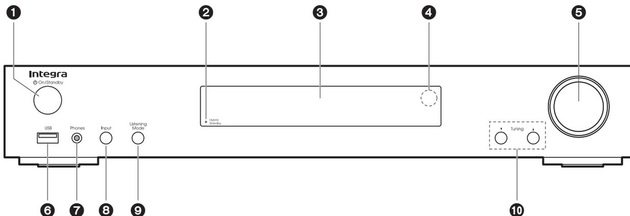
1. On/Standby button: Turns the unit on or into standby mode.
