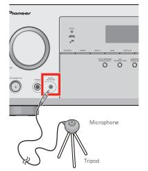
If you have a tripod, use it to place the microphone so that it's about ear level at your normal listening position. Otherwise, place the microphone at ear level using a table or a chair.
