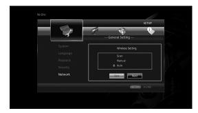
**Scan:** Select this option to search for available wireless networks. When the network list is displayed, select the SSID to be connected and enter the password.
