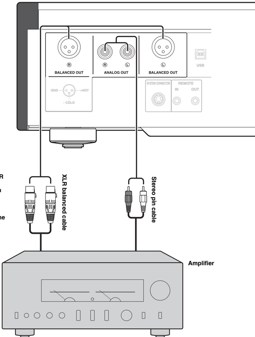
If your amplifier is equipped with XLR balanced input jacks, we recommend balanced connection for optimum audio performance.
