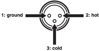
When connecting, be sure to match the pins and insert the connector of the "female" XLR balanced cable. When disconnecting, pull out the "female" XLR balanced cable while pressing down the latch lock on the plug.
