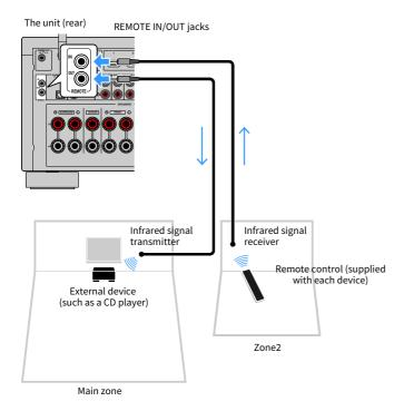
An infrared signal transmitter is not required if you are using Yamaha products that support remote connections, as the unit does. You can transmit remote control signals by connecting the REMOTE IN/OUT jacks with monaural mini-jack cables and an infrared signal receiver.
