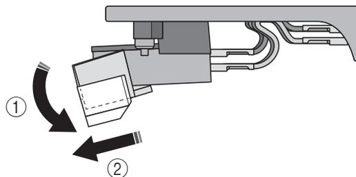
3 While using your fingers to hold the body of the cartridge, insert the tab of the replacement stylus into the groove on the underside of the cartridge.
