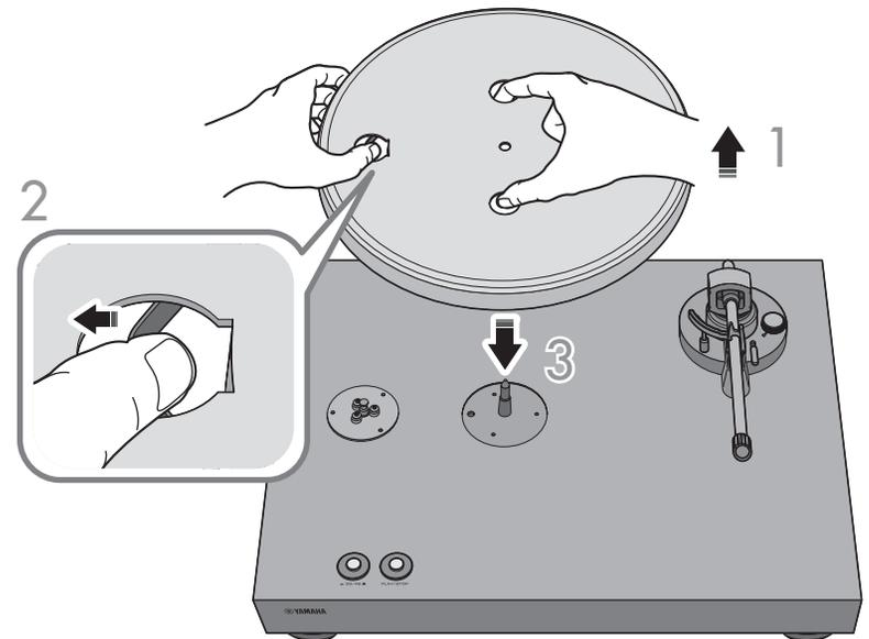
**4** Align the round hole of the platter with the pulley.
