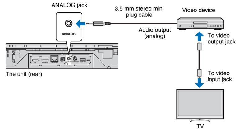
TV audio can be played through this unit by switching input to ANALOG using the ANALOG key on the remote control.
