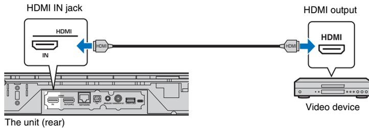
TV audio can be played through this unit by switching input to HDMI using the HDMI key on the remote control.
