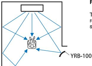
Figure 3. With a sound reflection board installed
