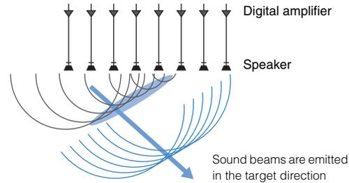
When these focused sounds hit a hard wall, they are reflected off of the wall. A digital sound projector outputs sound beams from five channels, including front (left/right), center, and surround (left/right) channels, by reflecting these beams off of walls so that sounds reach the listener from the appropriate direction. It features a technology that enables true surround sound without requiring the installation of speakers in front of, or behind, the listener.
