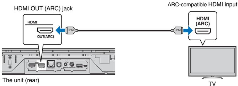
When connecting a TV that supports Audio Return Channel (ARC), enable the HDMI control function (p. 51).
