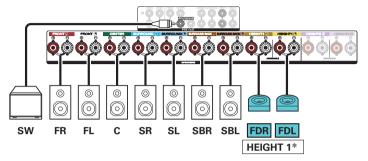
\* The surround Dolby or back Dolby speakers can be connected instead of the front Dolby speakers. In this case, set the Dolby Atmos Enabled speakers to be connected under "Height" - "Layout" in the menu. (12) p. 225)
