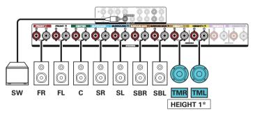
\* The top front or top rear speakers can be connected instead of the top middle speakers. In this case, set the ceiling speakers to be connected under "Height" - "Layout" in the menu. ( \*\*P p. 225)
