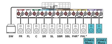
\* The height speakers, ceiling speakers and Dolby Atmos Enabled speakers can be connected to the HEIGHT1 speaker terminals. Set the speaker to be connected from "Height" - "Layout" in the menu. (12 p. 225)
