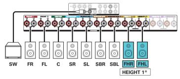
\* The rear height speakers can be connected instead of the front height speakers. In this case, set the height speakers to be connected under "Height" - "Layout" in the menu. (1287 p. 225)
