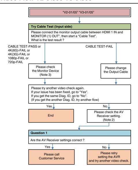
**Description "V\*-01"**: Miscommunication with Monitor at output terminal (HPD always low).
