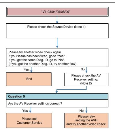
**Description "V1-03"**: Cannot detect the HDMI signal from the source device at the AVR input terminal (TMDS Rx PLL Lock, but SCDT(CKDT) OFF).
