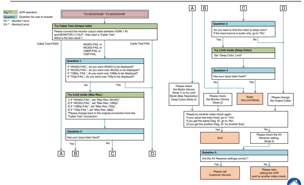
**Description "V\*-02"**: Miscommunication with Monitor at output terminal (4K60 output setting error).
