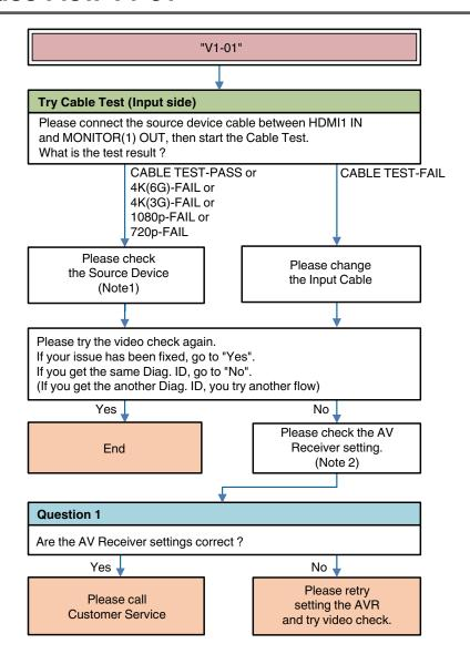
**Description "V1-01"**: Cannot detect the HDMI cable connected to the AVR input terminal (as detection of 5V from Source Device).
